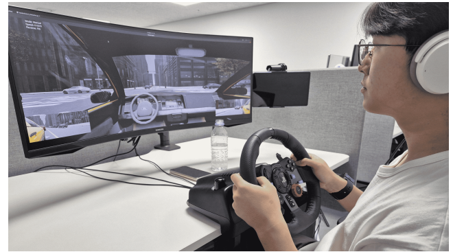
Figure 2: User study setup. The custom driving simulator consists of a 38-inch curved monitor, a Logitech G29 steering wheel and pedal set, and a Galaxy Tab S6 Lite tablet used to present video-based NDRTs. Participants received TORs through a Sennheiser Accentum wired headset while driving in CARLA. A custom smartwatch worn on the right wrist provided IMU and PPG signals for biometric acquisition.
